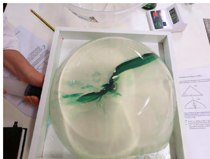
Carrying out gelatine-based experiments of fluid-filled crack propagation in elastic media during the analogue modelling workshop on the first day
